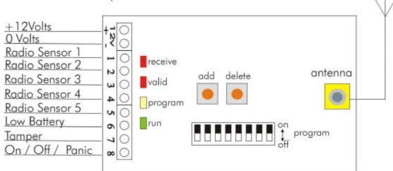
Receive: On when any data packets are received
